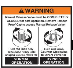
MANUAL RELEASE VALVE PROCEDURE DECAL LOCATED ON THE INSIDE OF THE PROTECTIVE CAP
